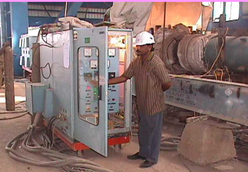
WELDING SEGMENT BALANCE TIME IN PROGRAMMER MADE TO ZERO AFTER COMPLETION OF WELDING
