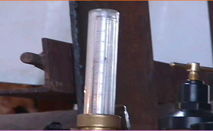
ARGON PURGING STARTED AT 25 lpm
