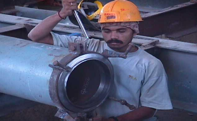
MECHANICAL PIPE CLAMP BEING FIXED ON PIPE FOR JOINT FITUP
