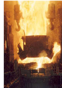
2 - Melting in the ultra-high power electric furnace
