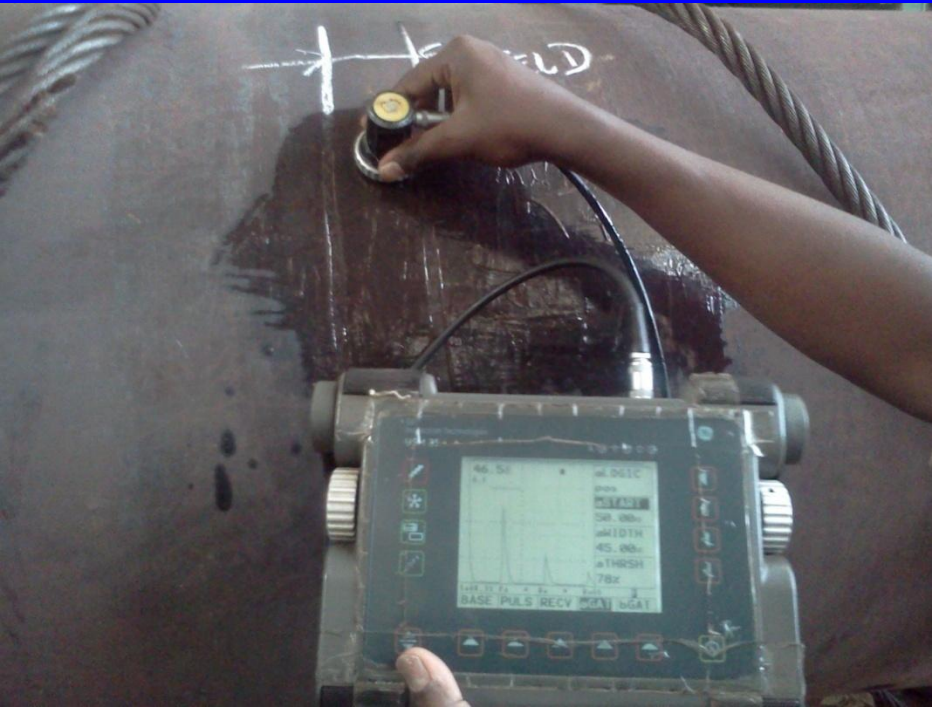
Normal beam scanning of header butt welds
