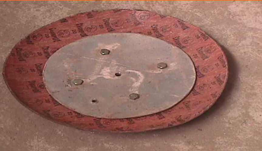
GASKET WITH ALUMINIUM SHEET FOR ARGON PURGING DAMPER ARRANGEMENT
