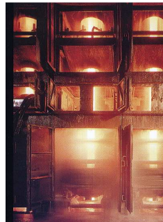
4 - A bowtype continuous casting plant has replaced the old vertical rotary caster
