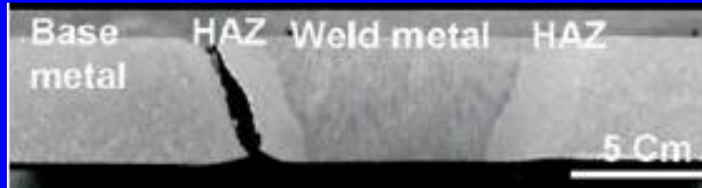
Type IV Failure in Weld joint
