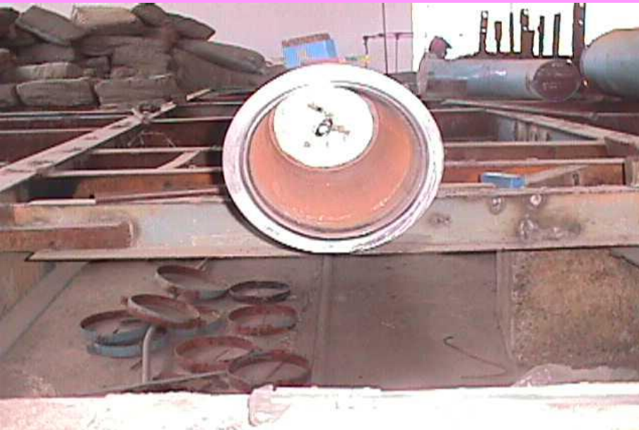
ARGON PURGING DAMPER ARRANGEMENT FIXED INSIDE THE PIPE
