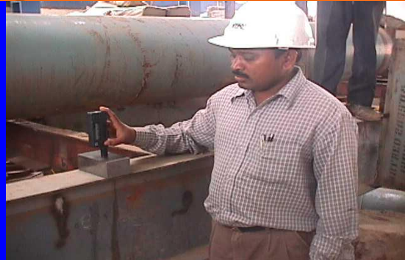
HARDNESS TESTER USED TO MEASURE CORRECTION FACTOR
