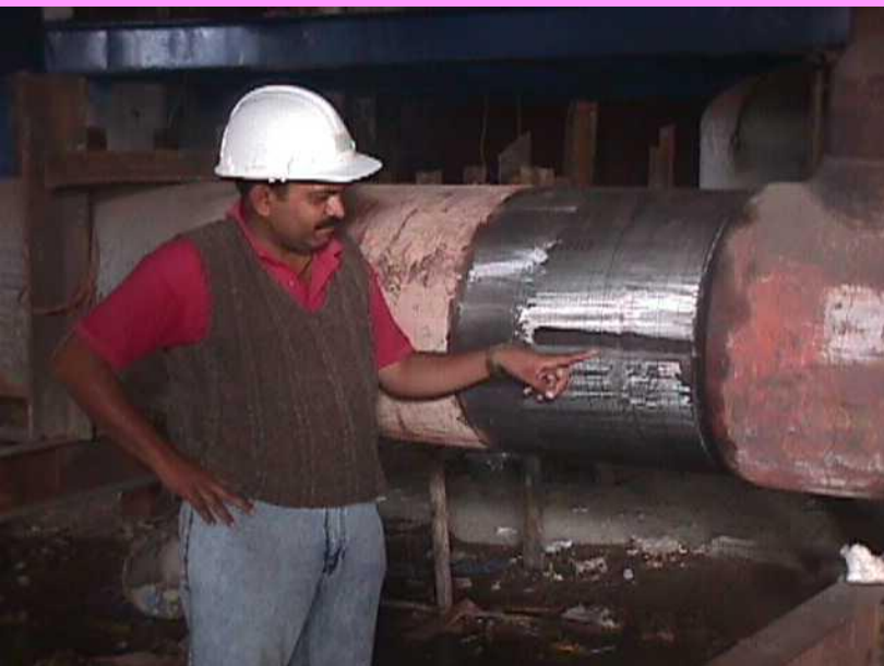
WELD SURFACE FLUSH GROUND FOR NDE
