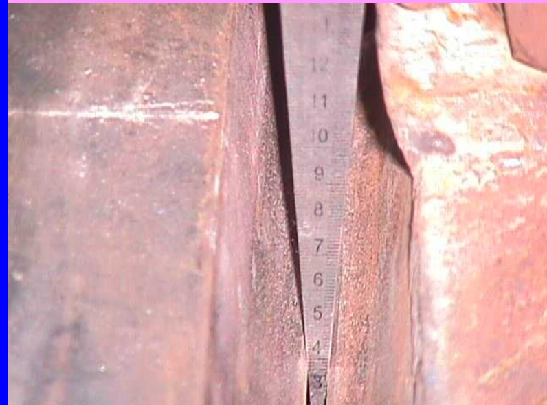
JOINT ROOT GAP CHECKED USING TAPER GAUGE
