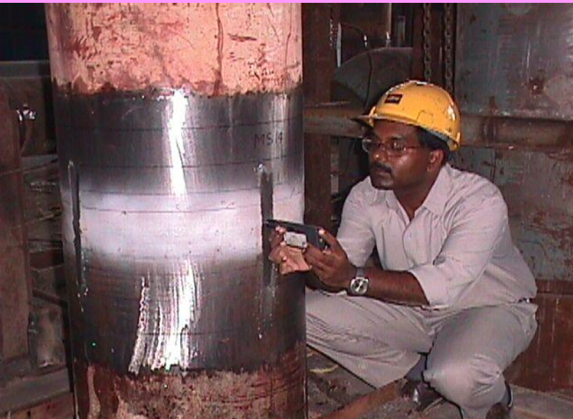
HARDNESS TESTER USED TO MEASURE HARDNESS VALUE ON THE PIPE
