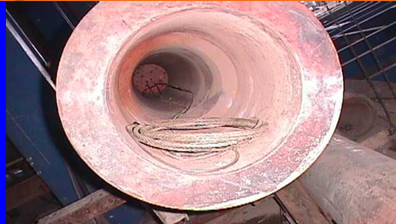
WIRE ROPE ARRANGEMENT FOR PULLING OUT DAMPERS AFTER COMPLETION OF TWO PASS SMAW
